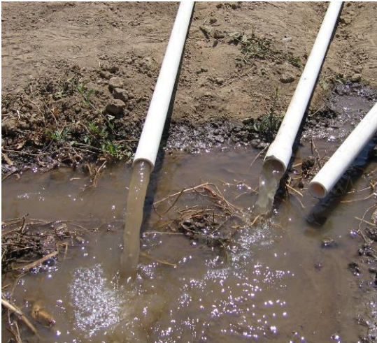
Figure 2. Photograph demonstrating visual difference between untreated and PAM treated runoff: water on left from untreated furrow, water on right from furrow treated with PAM
