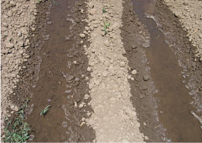
Figure 1. Photograph demonstrating visual difference between untreated and PAM treated runoff: left furrow treated with PAM, right furrow untreated
