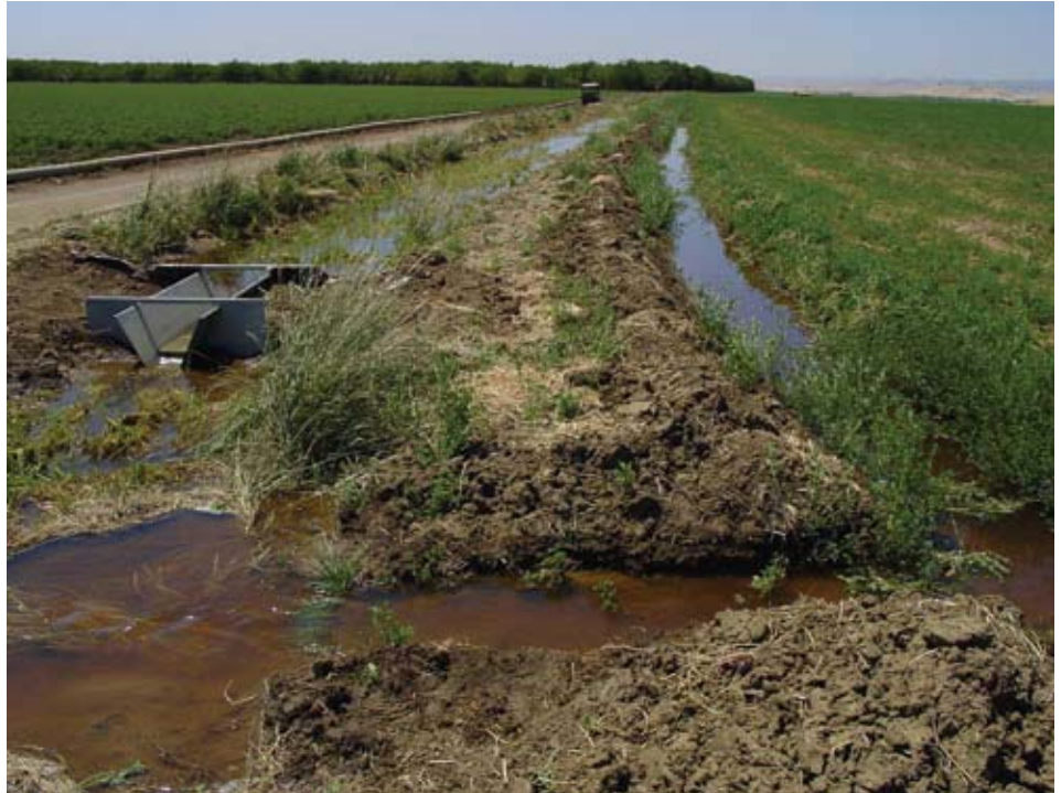
The ditch on the left is a vegetated ditch and the ditch on the right is a standard dirt ditch (no vegetation). The velocity of runoff from the alfalfa field is significantly reduced in the vegetated ditch. This alfalfa field and the two ditches were used for a vegetated ditch study and the Landguard studies.
